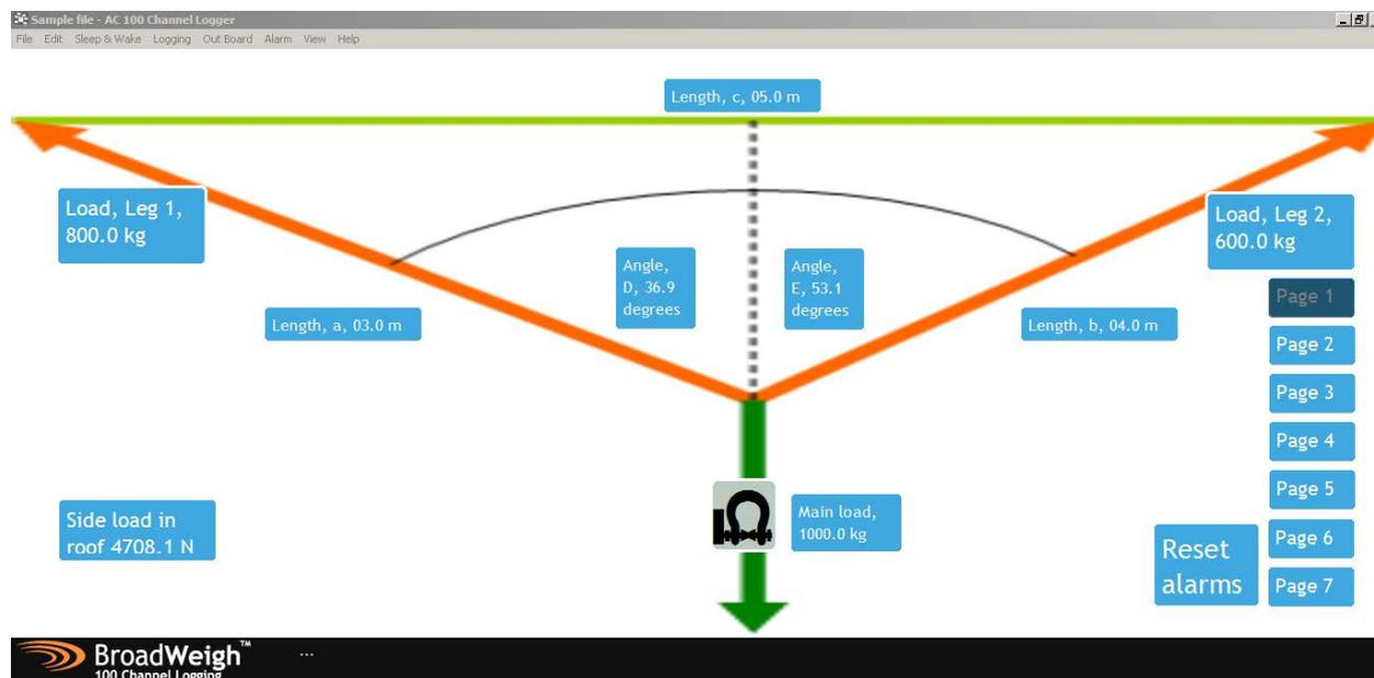
This page shows the load in the legs of a two-leg bridle. It is based on the load cell on channel 1 and the lengths a, b and c which are entered into LOG 100 channels 4, 5 and 6.
