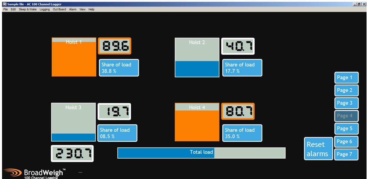
This shows a graphical and numeric representation of the loads on four theoretical hoists. We are also displaying the percent share of the total load on each hoist. There is also a bar and display for the total load. Alarms set at 80 (warning) and 99 (overload).
