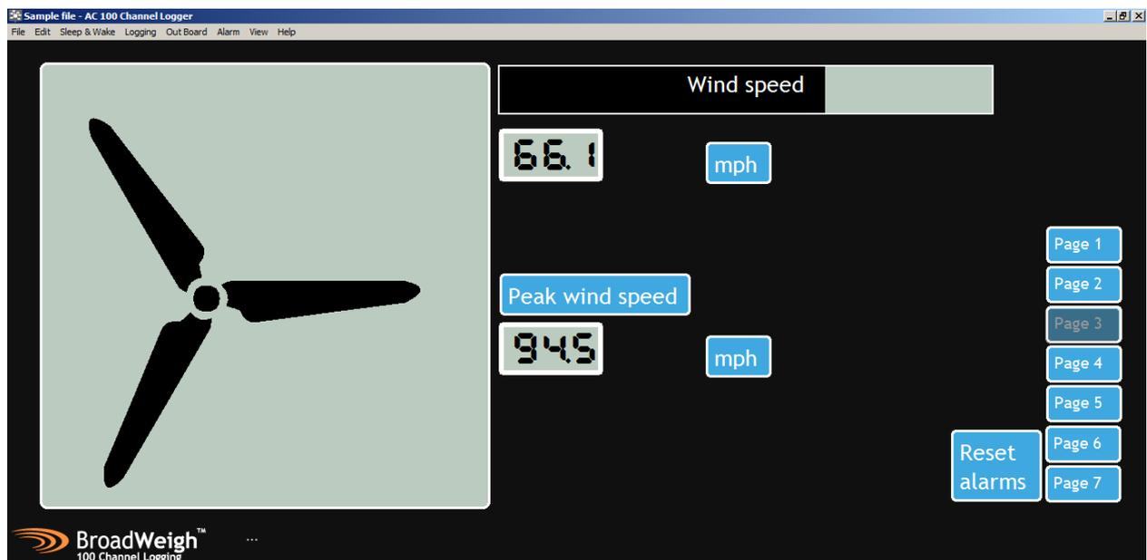
This page shows a method of displaying data from a WSS Wind Speed Sensor. The source for this is a SIM channel with heavy filtration to make it look a little more like real data. Alarms are set at 70 (warning) and 90 (overload).
