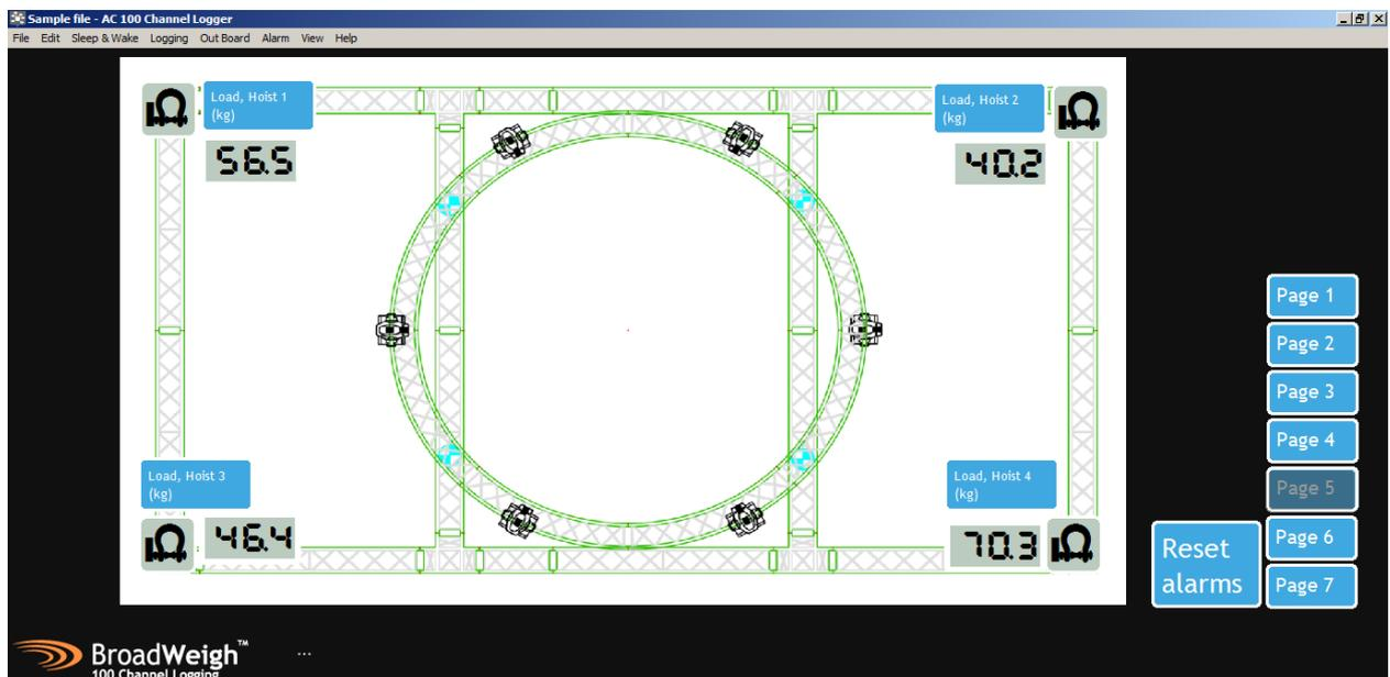
Similar to page 4 but just displayed on a plan with no bar graphs. Also note that the shackle icons are linked to the relevant channel's data and therefore warnings and alarms.
