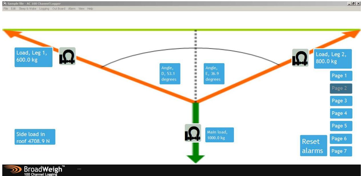
As a check for the previous page we made this page with the load cells in the legs as well. Interestingly, we found at PLASA that it didn't quite add up. Using relatively low loads the amount of twist in the bridle leg and manufacturing tolerances meant that even with an apparently even load (2m per leg) the load was not evenly distributed.
