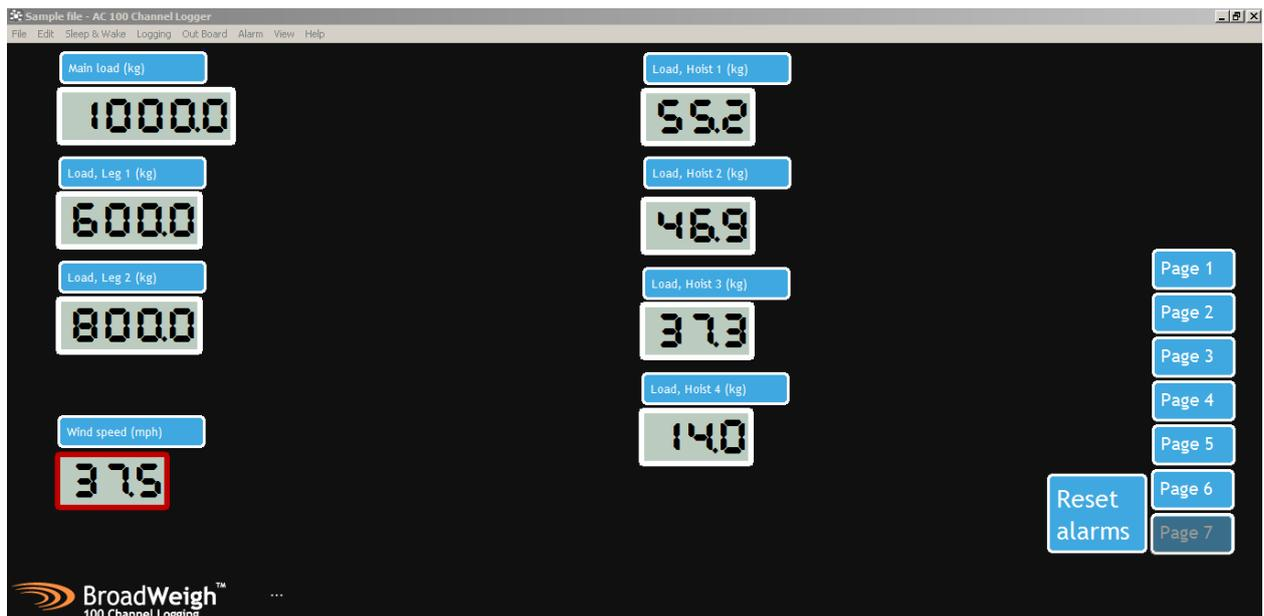
There are a lot of data channels on the main page making it difficult to see exactly what you want to. Here we have just put the main 8 data channels in an easy to read display. In this format we can put the channels in any order, anywhere on the page giving real flexibility.
